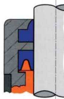
Thorwiper groove mounted in the gland or stuffing box.
