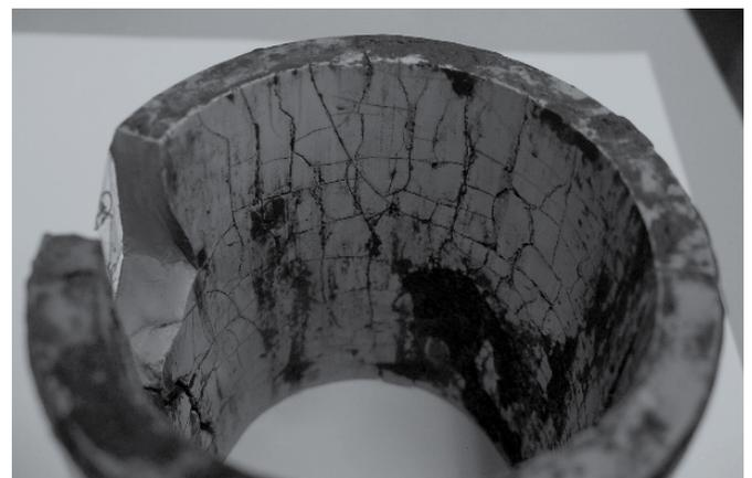
*Typical example of ThorPlas bearing with hydrolysis.*
