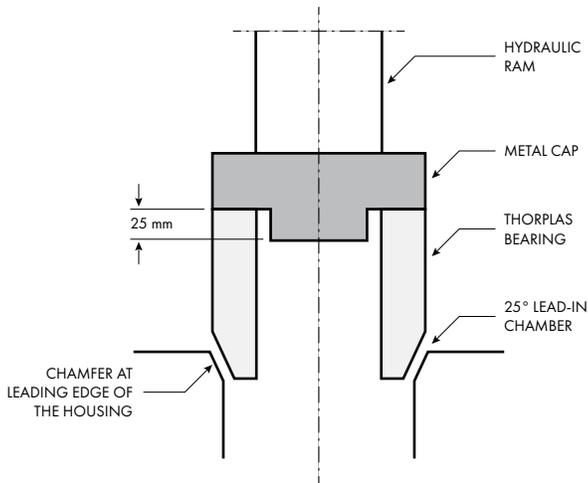
Figure 17: Press in set up for ThorPlas bearings
