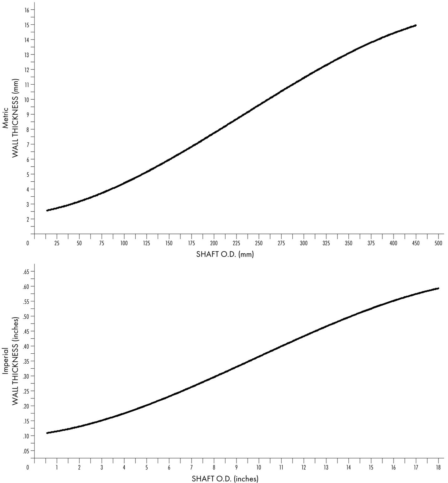
**Figure 8: Typical ThorPlas Minimum Wall Thickness Guide**
