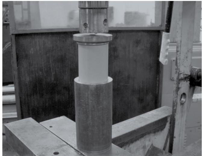
2) 75% of bearing length inside the housing.
