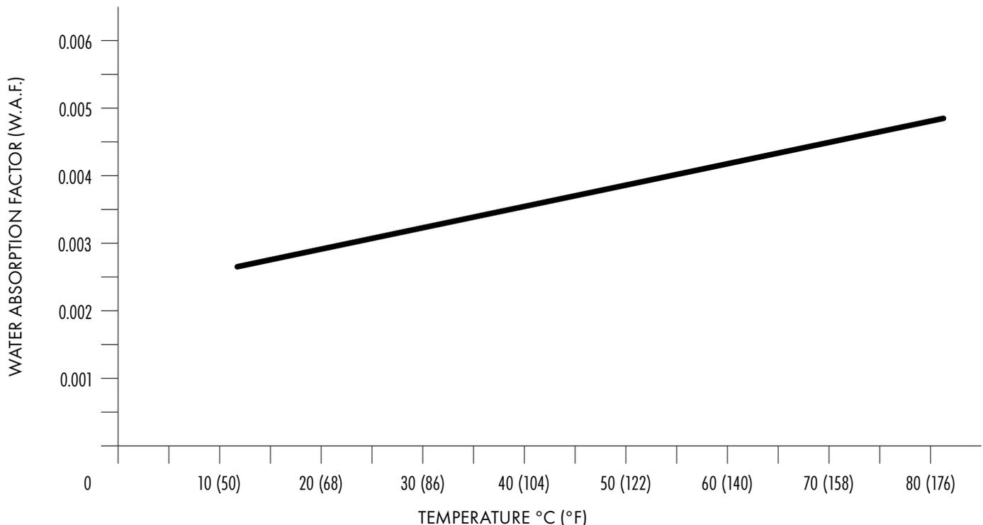
Figure 11: Typical Water Absorption Factor (W.A.F.) for Various Water Temperatures
